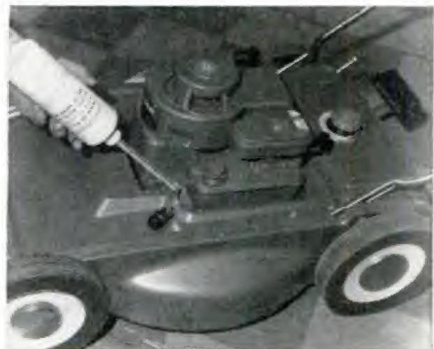
FOUR-CYCLE ENGINE OIL is critical in preventing cylinder scoring. Use what manufacturer suggests
